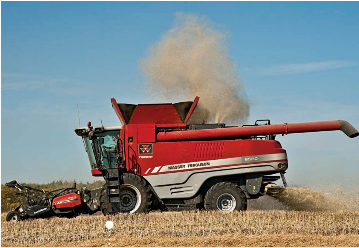
ABOVE: The V-Cool fan in reverse mode clears the intake screen. RIGHT: Dean Sleezer prepares to switch a section of the new, smaller interchangeable concave.
