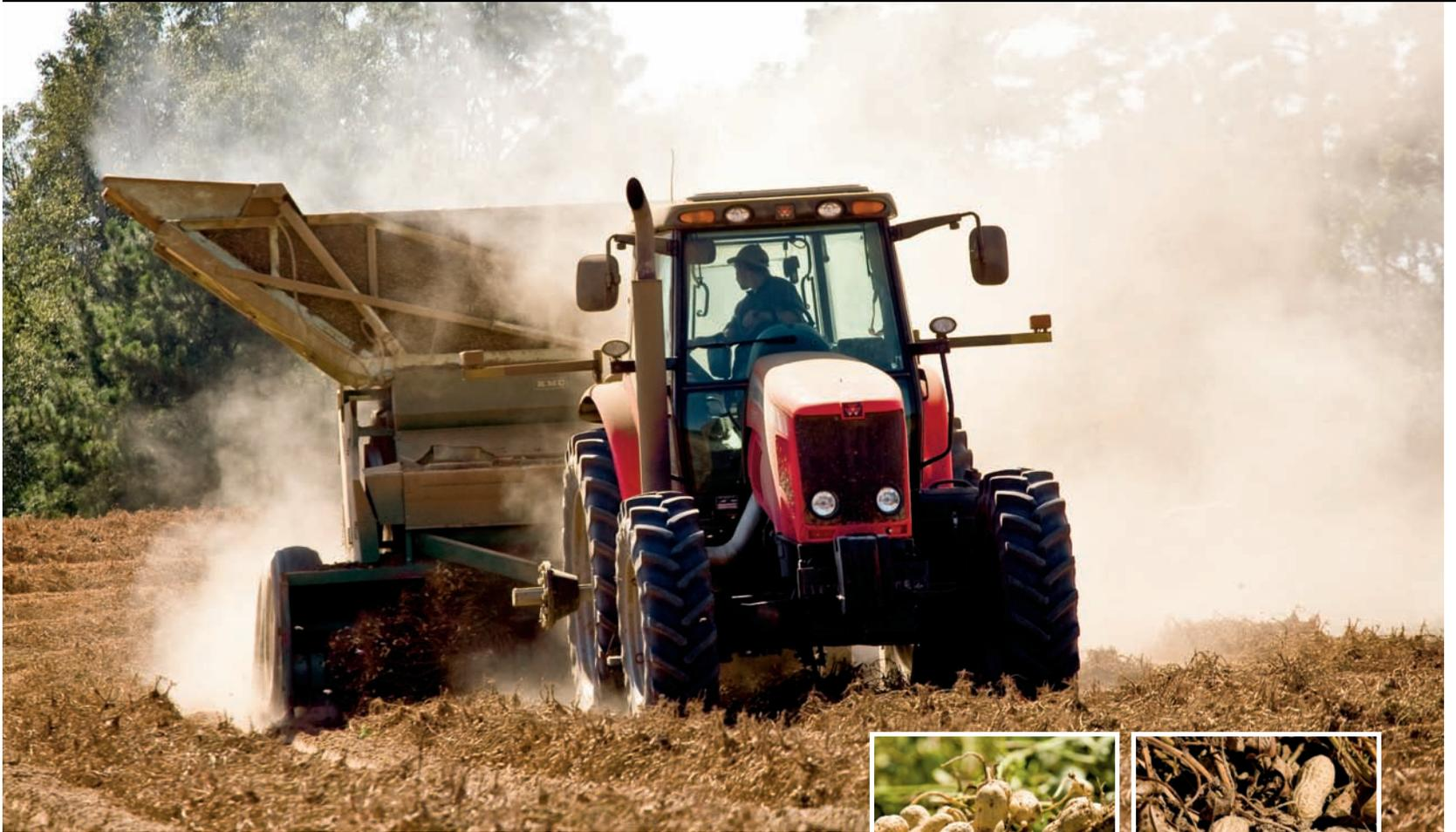
Now, the spring tooth header reel on the front of each combine gobbles up the two windrows. As the plants disappear into the maw of the machine, the decibel count mounts as the pods are separated from the plants. The peanuts are carried into a 2-ton-capacity basket on the combine, while the stalks and leaves are spit out of the back of the combine.
